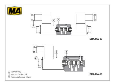
On/off direct and pilot operated directional valves equipped with explosion-proof solenoids certified according to **MA** Chinese mining certification, protection mode:
