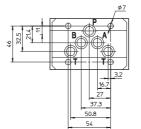
= PRESSURE PORT A, B = USE PORT T = TANK PORT
